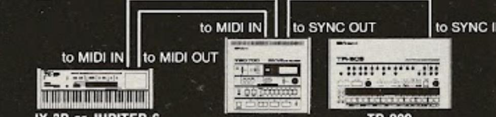
The sound sources of the TR-909 can be played using the keys of the PIANO PLUS 400. The volume changes depending on how forcefully the key is touched.
